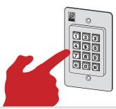
Secure keypad unit to junction box using either set of included screws. (Gasket is optional if mounted indoors.)
