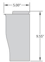
Hole pattern on back for pedestal mounting is spaced at 3.063" with pilot holes for alternate mounting at 2.5".
