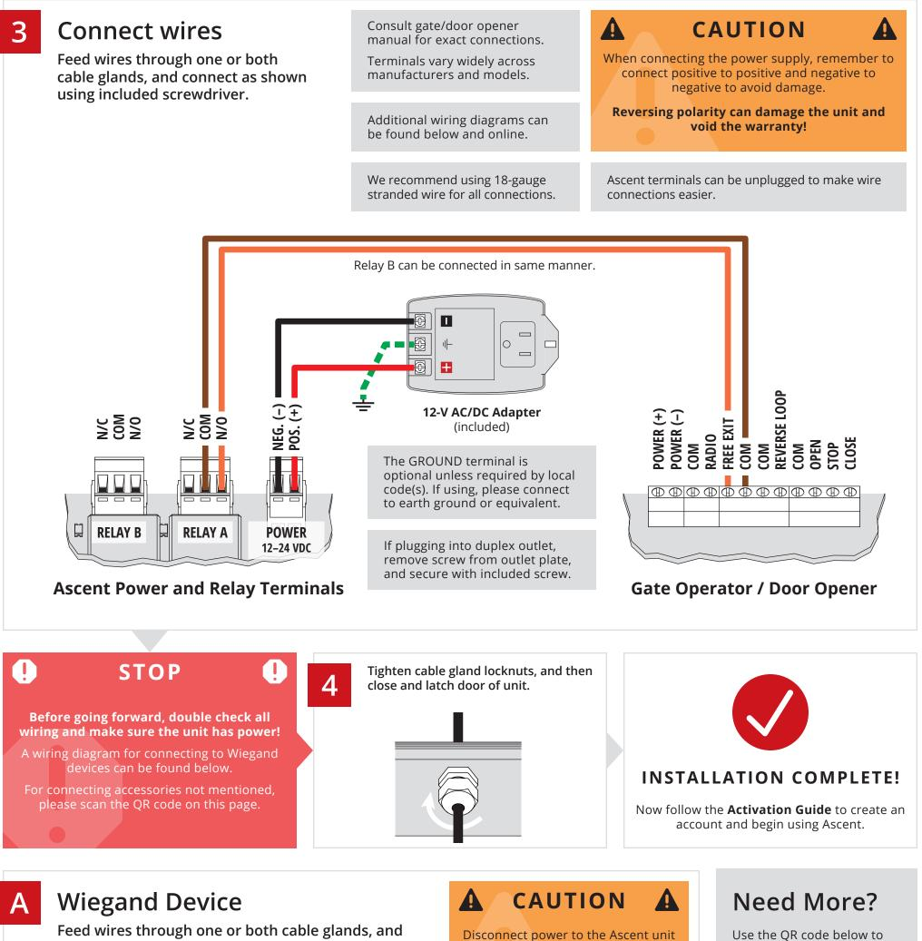
**connect as shown using included screwdriver.** These terminals are used to connect a Wiegand device such as a card reader or Wiegand keypad. before connecting Wiegand devices.
