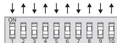
DIP Switches on Receiver 300 (default positions)
