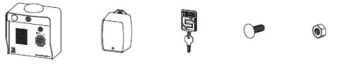
Ascent Unit    12-V AC/DC Adapter (PS-12DC1)    Key    Carriage Bolt (4x)    Hex Nut (4x)
