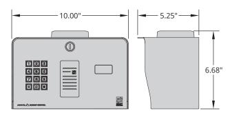
Hole pattern on back for pedestal mounting is spaced at 3.063" with pilot holes for alternate mounting at 2.5".
